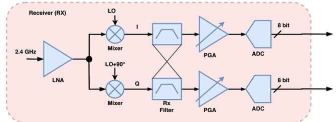
Fig. 1 Low-IF Receiver for a BLE System.
