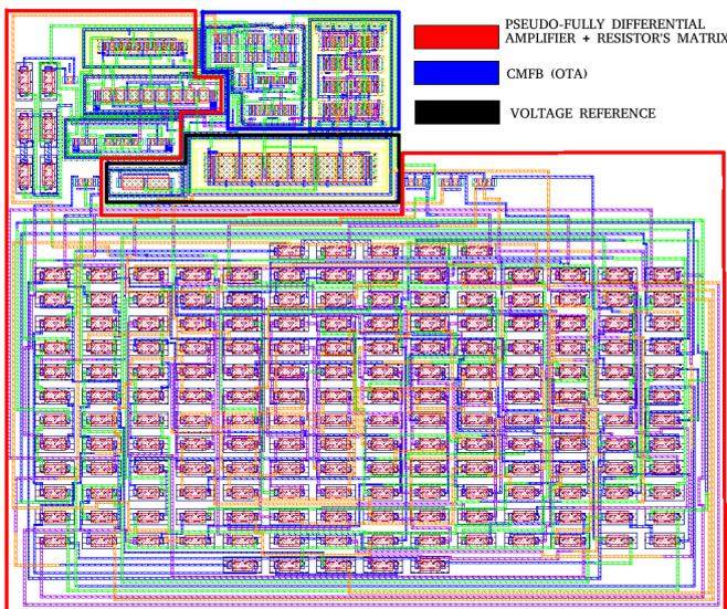
Fig. 6 Layout of PGA
