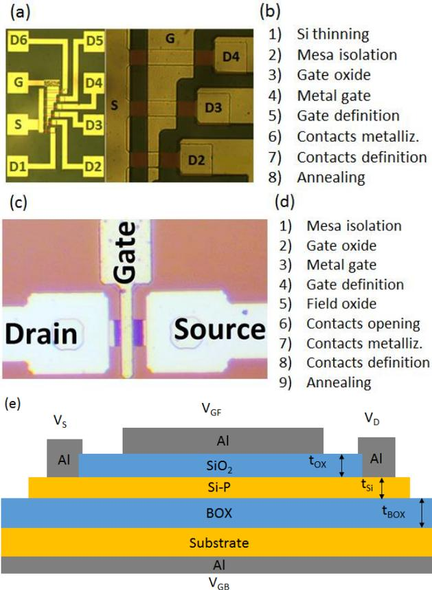
Fig. 1 (a) Picture of an L-array and (b) its fabrication steps of the <sup>BE</sup>SOI MOSFET. (c) Picture of an isolated transistor and (d) its fabrication steps of the UTBB <sup>BE</sup>SOI MOSFET. (e) schematic cross-section of the <sup>BE</sup>SOI MOSFET
