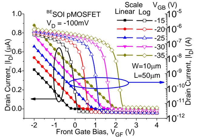
Fig. 2 Transfer characteristics ( $I_D(V_{GF})$ ) of the <sup>BE</sup>SOI transistor for different back gate bias ( $V_{GB}$ ) in linear (left) and log-scale (right).
