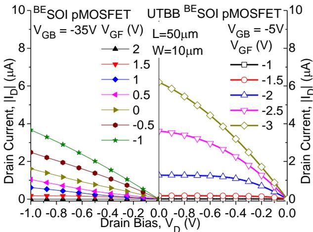
Fig.9 Output characteristics ( $I_D(V_D)$ ) of the BE SOI (left) and UTBB BE SOI transistor (right) for different  $V_{GF}$ .
