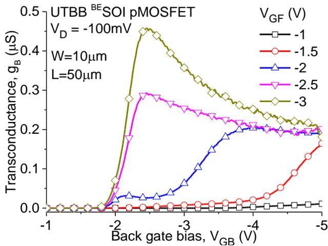
Fig.8 Transconductance related to the  $V_{GB}$  ( $g_B$ ) of the UTBB BE SOI during the  $V_{GB}$  sweep for various  $V_{GF}$ .
