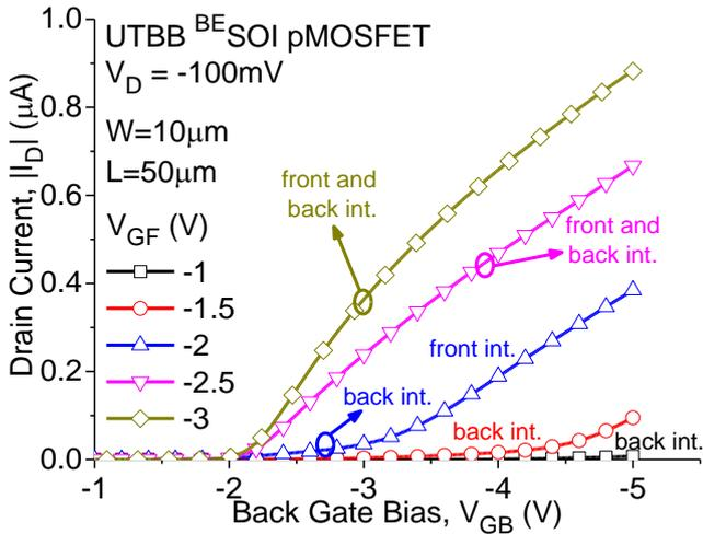
Fig. 5 Drain current in linear scale as a function of the back gate bias ( $I_D(V_{GB})$ ) of the UTBB <sup>BE</sup>SOI transistor for various front gate bias ( $V_{GF}$ ).
