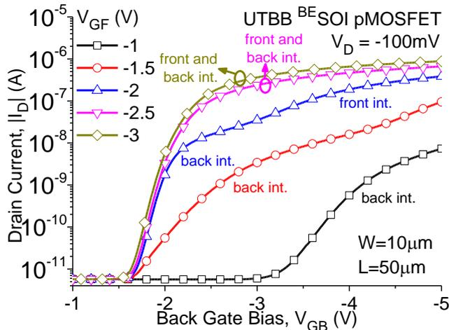
Fig. 6 Drain current in log scale as a function of the back-gate bias ( $I_D(V_{GB})$ ) of the UTBB <sup>BE</sup>SOI transistor for various front gate bias ( $V_{GF}$ ).
