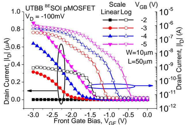
Fig. 3 Transfer characteristics ( $I_D(V_{GF})$ ) of the UTBB <sup>BE</sup>SOI transistor for different back gate bias ( $V_{GB}$ ) in linear (left) and log-scale (right).
