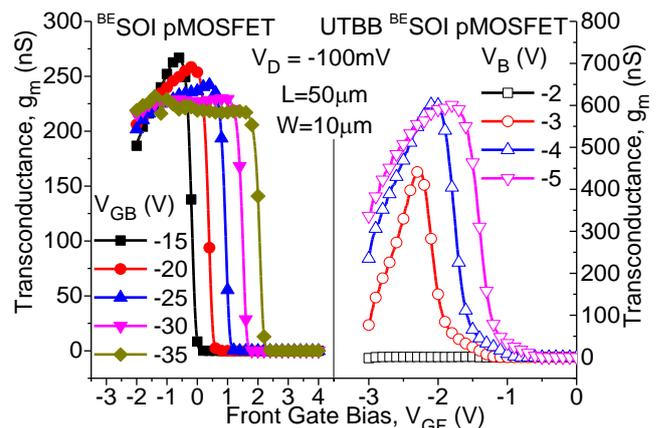
Fig. 7 Transconductance of the <sup>BE</sup>SOI (left) and UTBB <sup>BE</sup>SOI (right) transistor during the  $V_{GF}$  sweep for various  $V_{GB}$ .
