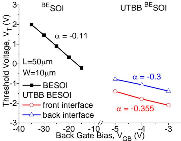
Fig.4 Threshold voltage as a function of the back gate bias of the  $^{BE}SOI$  transistor (left) and  $UTBB^{BE}SOI$  (right).
