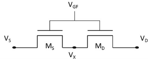
Fig. 1 - Schematic representation of a self-cascode transistor.
