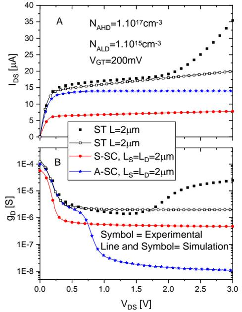
Fig. 4 - (A) Drain current and (B) output conductance as a function of drain voltage measured for single transistor, symmetric and asymmetric self-cascode devices, biased at  $V_{GT} = 200$  mV.
