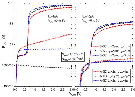
Fig. 9 -  $R_{OUT}$  curves as a function of  $V_{OUT}$ , biased at  $I_{IN} = 1 \mu A$  and  $I_{IN} = 10 \mu A$  for CMs implemented with symmetric and asymmetric self-cascode structure with  $L_S$  fixed varying  $L_D$  from  $1 \mu m$  to  $3 \mu m$ .
