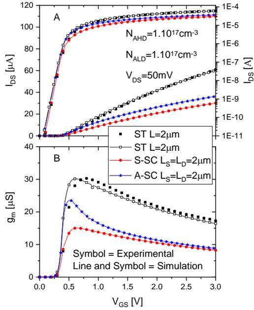
Fig. 3 - (A) Drain current and (B) transconductance as a function of gate voltage measured for single transistor, symmetric and asymmetric self-cascode devices, biased at  $V_{DS} = 50$  mV.
