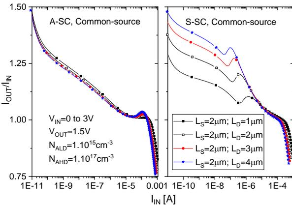
Fig. 7 -  $I_{OUT}/I_{IN}$  curves as a function of input current for CMs implemented with ST, S-SC and A-SC transistors with  $L_S$  fixed and  $L_D$  variable, simulated at  $V_{OUT} = 1.5\text{V}$ .
