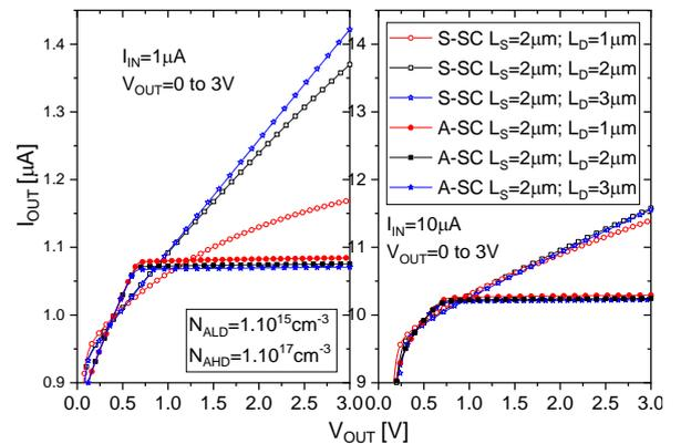
Fig. 8 -  $I_{OUT}$  curves as a function of  $V_{OUT}$ , biased at  $I_{IN} = 1 \text{ }\mu\text{A}$  and  $I_{IN} = 10 \text{ }\mu\text{A}$  for CMs implemented with symmetric and asymmetric self-cascode structure with  $L_S$  fixed varying  $L_D$  from  $1 \text{ }\mu\text{m}$  to  $3 \text{ }\mu\text{m}$ .
