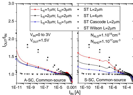
Fig. 5 -  $I_{OUT}/I_{IN}$  curves as a function of input current for current mirrors implemented with conventional transistors in common-source, Cascode and Wilson architecture, symmetric and asymmetric self-cascode, extracted at  $V_{IN} = 0$  V -  $3$  V and  $V_{OUT} = 1.5$  V.
