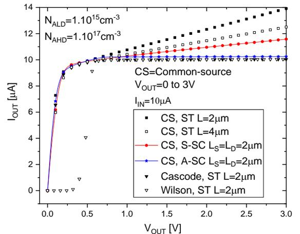
Fig. 6 -  $I_{OUT}$  curves as a function of the output voltage, biased at  $I_{IN} = 10 \mu\text{A}$  for current mirrors implemented with conventional transistors in common-source, Cascode and Wilson architecture, symmetric and asymmetric self-cascode structure.
