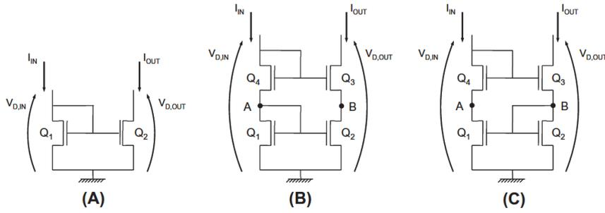
Fig. 2 - Common-source (A), Cascode (B), and Wilson (C) current mirrors architectures.
