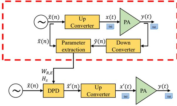
Fig. 10 Setup for the PA model extraction (red dashed rectangle) and its use in a DPD unit.
