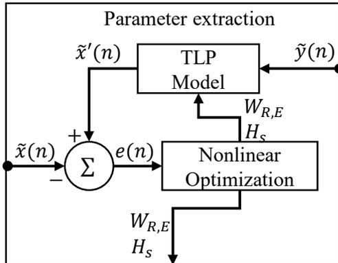
Fig. 11 A detailed description of the parameter extraction block defined in Fig. 10.
