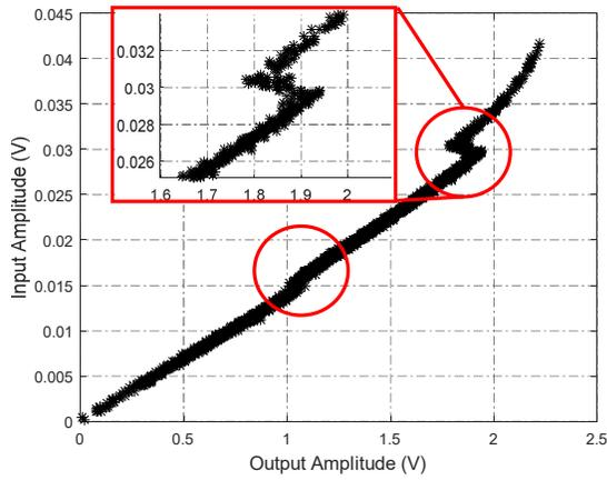
Fig.7 Overlapping of amplitude samples on multimode PA AM-AM inverse behavior.
