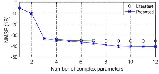
Fig. 12 NMSE in function of number of complex-valued parameters for the literature and proposed models with ascendant method. The maximum number of parameters is set to 12.
