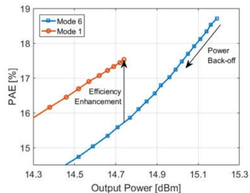
Fig.2 Measured PAE vs. output power.
