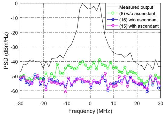
Fig.13 Power spectral densities (PSDs) of the measured output and of the error signals in function of frequency for the TLP-based models been analyzed. The w/o ascendant indicates without ascendant. All models present 36 complex-valued network parameters.
