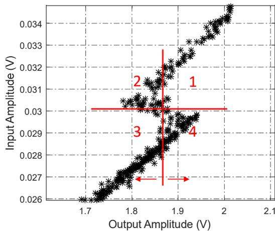
Fig.8 Detailed overlapping samples for the transition between the two modes with higher amplitudes. The vertical line sweeps the values until the  $L_3$  that minimizes the excluded samples is found. The samples to be excluded are in the even quadrants.
