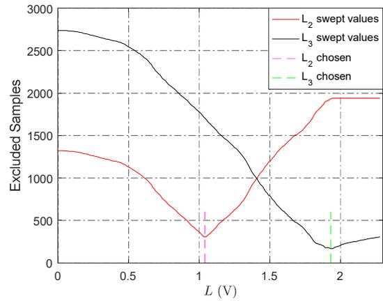
Fig.9 Variation of  $L_2$  in relation to excluded samples with  $L_3$  fixed. Variation of  $L_3$  in relation to excluded samples with  $L_2$  fixed. The valleys indicate the minimum amounts of excluded samples to the respective chosen limits.
