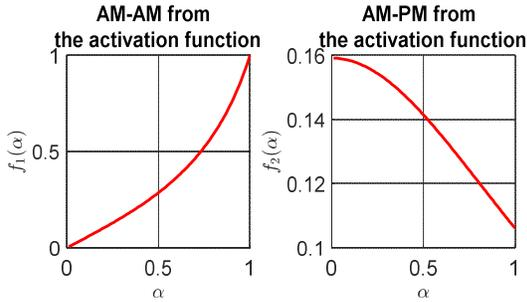
Fig.5 AM-AM and AM-PM characteristics of the proposed activation function of (15).  $\alpha$  is the argument of the activation function given by the amplitude of the complex-valued signal applied to the neuron input.  $f_1$  and  $f_2$  are the proposed functions.
