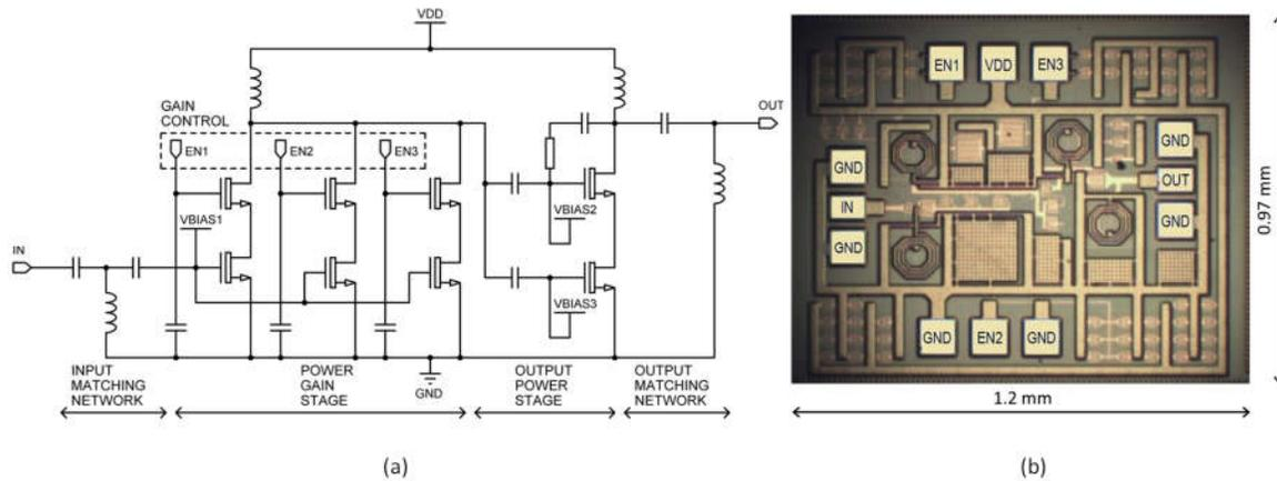
Fig.1 (a) Circuit topology of the PA (bias circuitry is omitted) and (b) chip micrograph of the PA.
