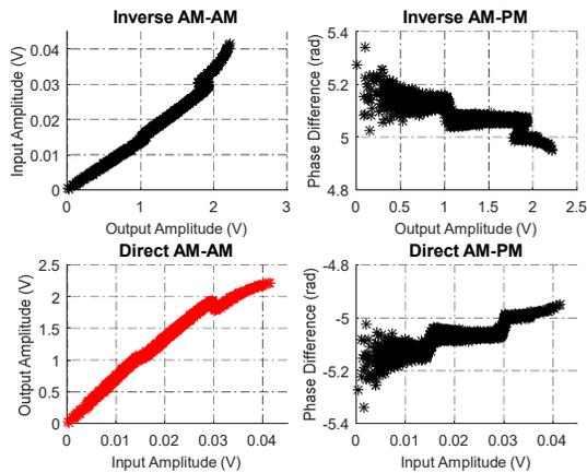
Fig.3 Simulated inverse and direct multimode PA transfer functions.
