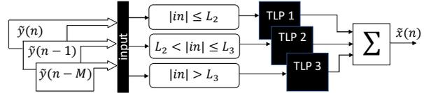
Fig.6 Diagram of the proposed TLP-based inverse model for the multimode PA with three modes.
