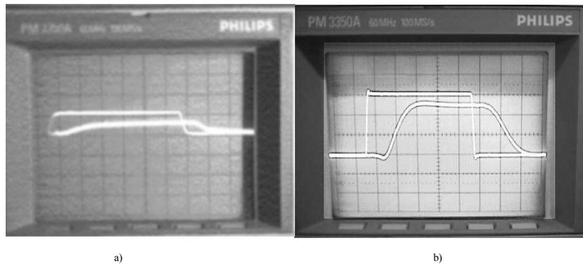
Fig. 9. Step response of the controller: a) Small amplitude input step ( $\Delta V_{in} = 500\text{mV}$ ). Vertical scales: input =  $0.5\text{V/div}$  - output =  $0.2\text{V/div}$ . Time scale:  $100\text{ ns/div}$ . b) Large amplitude input step ( $\Delta V_{in} = 3\text{V}$ ). Vertical scales: input =  $1\text{V/div}$  - output =  $0.2\text{V/div}$ . Time scale:  $200\text{ ns/div}$ .
