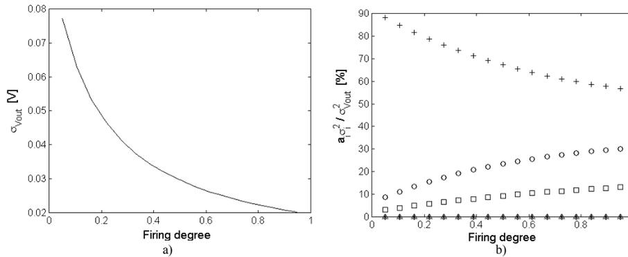
Fig. 6. a) Simulated  $\sigma_{Vout}$  with only one active rule as a function of the firing degree of the rule. b) Individual contribution of each building block to the total output variance: (+) divider; (o) consequent+D/A; (□) mirror before  $ID$ ; (◇) T-Norm; (△) CFMF and (\*)  $I_o$ .
