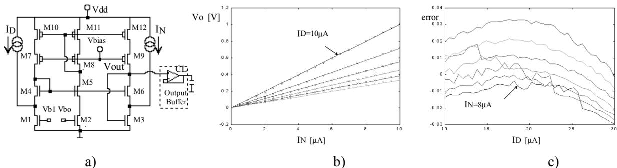
Fig.4. a) Transresistive divider circuit. b) Measured (x) and calculated (-)  $V_o$  for  $0 < I_N < 10 \mu A$  while  $I_D$  ranges from 10  $\mu A$  to 30  $\mu A$  by 4  $\mu A$  steps. c) Measured relative error of the divider.
