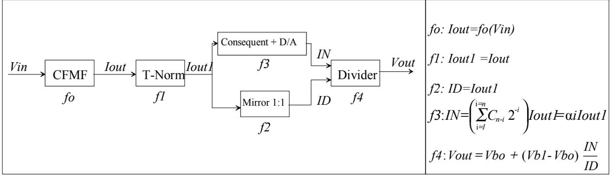
Fig.5. Simplified block diagram of the controller with only one fired rule for the estimation of the variance of its output  $V_{out}$ .
