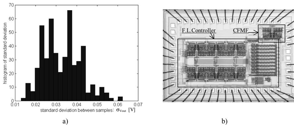
Fig. 10. a) Distribution of the Standard Deviation of the controller's output in the dc test from six measured samples. b) Microphotograph of the chip: Fuzzy Logic Controller and testing CFMF.
