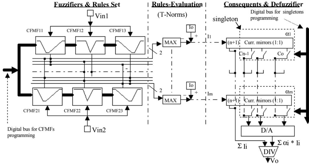
Fig. 1. Block diagram of the Zero-Order Takagi-Sugeno Fuzzy Logic Controller.
