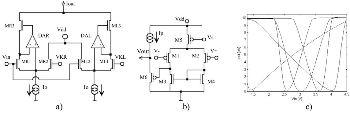
Fig. 2. a) Complementary Fuzzy Membership Function (CFMF) Circuit. b) Differential Amplifiers *DAL* *DAR*. c) Some measured transfer functions '*Iout* vs. *Vin*' of the CFMF using a HP4145B instrument.
