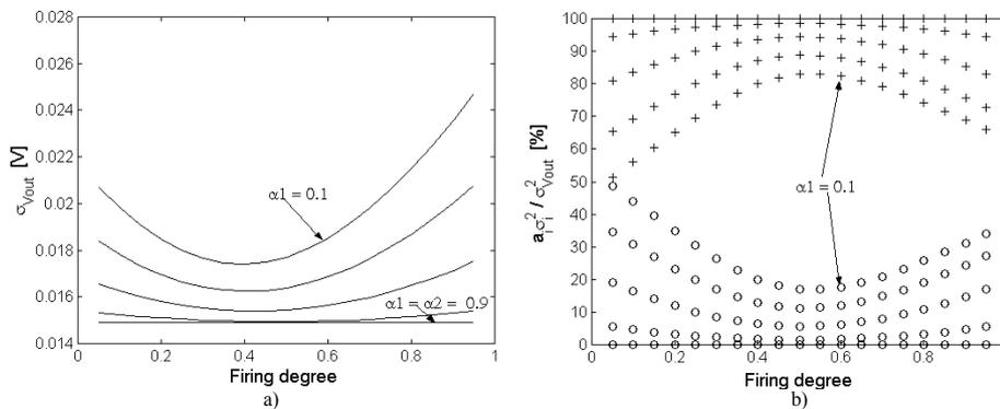
Fig. 7. a) Simulated  $\sigma_{Vout}$  assuming two rules fired in a complementary way. The singleton of one rule ( $\alpha_2$ ) was set to 0.9. In the other rule the singleton ( $\alpha_1$ ) ranges parametrically from 0.1 to 0.9. b) Individual contributions to the total output variance for different values of the singleton  $\alpha_1$ : (o) CFMF+T-Norm+ $I_o$  and (+) divider.
