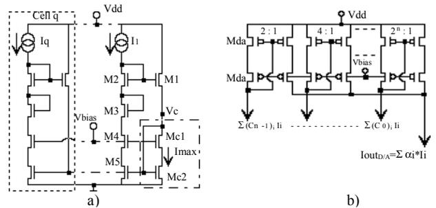
Fig. 3. a) Multiple-Input MAXIMUM circuit, b) Weighting D/A circuit.
