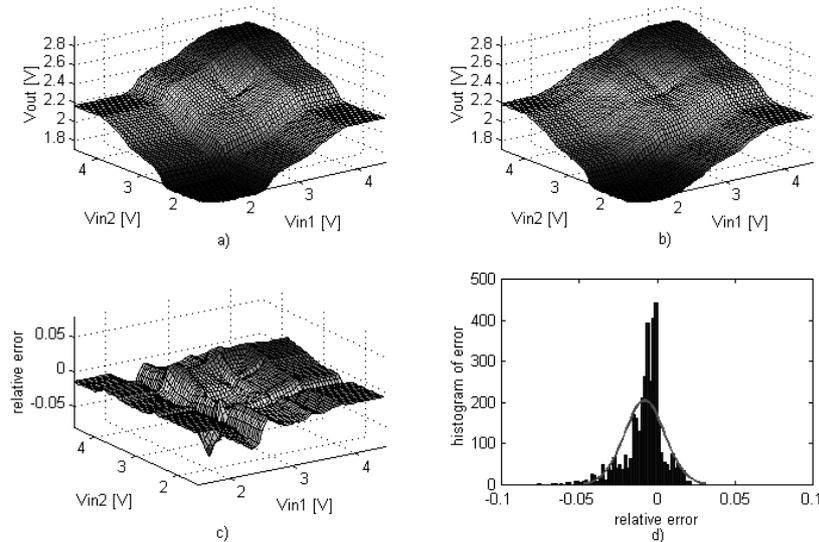
Fig. 8. dc test results: a) Simulated output surface. b) Measured output surface. c) Measured relative error surface. d) Relative error distribution.
