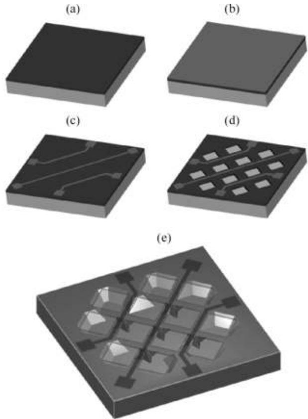
**Figure 1.** Step sequence to produce the Si microtips : (a) Deposition of  $1.8\ \mu\text{m}$  thick PECVD  $\text{SiO}_x\text{N}_y$  film and (b) of a  $3500\ \text{\AA}$  film of chromium. (c) Patterning of the electrode geometry. (d) Square holes (inclined  $45^\circ$ ) are opened in the  $\text{SiO}_x\text{N}_y$  film. (e) Anisotropic wet etching of Si in KOH solution to form the microtips.
