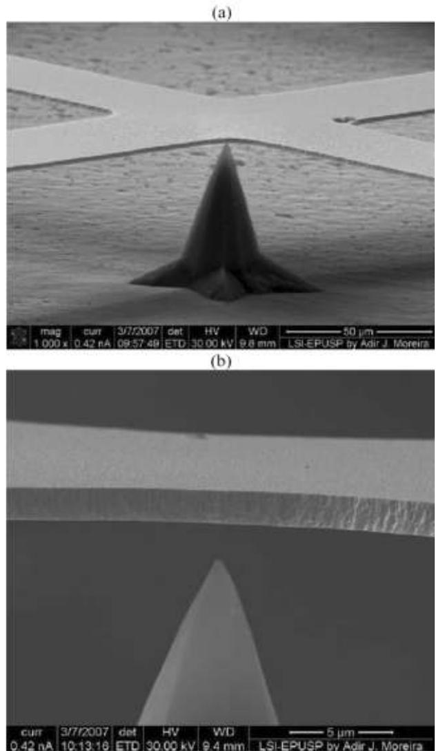
**Figure 7.** Close-up of a microtip as observed from a SEM. (a) The typical height of the tips is ~52 µm and the diameter at the vertex is below 1 µm. (b) The distance between the apex of the tips and the SiO<sub>x</sub>N<sub>y</sub> film is lower than 5 µm.
