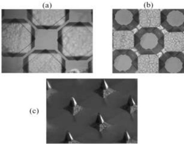
**Figure 5.** Top view of the microtips in the (a) first and (b) second stages of formation. In (c) a 3D image of the tips after the third stage (note that the SiO<sub>x</sub>N<sub>y</sub> grid was removed to better visualize the tips geometry).
