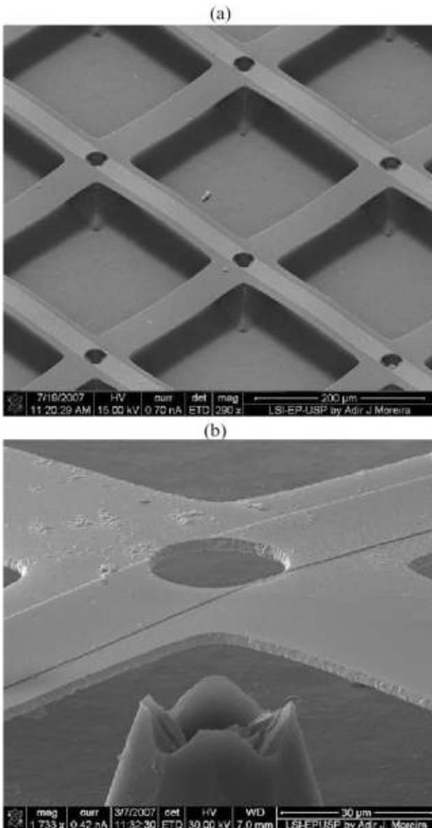
**Figure10.** (a) Removed Cr disks from the electrode lines on the top of the tips, leading to the loss of the electrode near the tip apex. (b) Undesired corrosion of top of the Si tips through the circular hole in the Cr electrode. Images from a scanning electron microscope (SEM).
