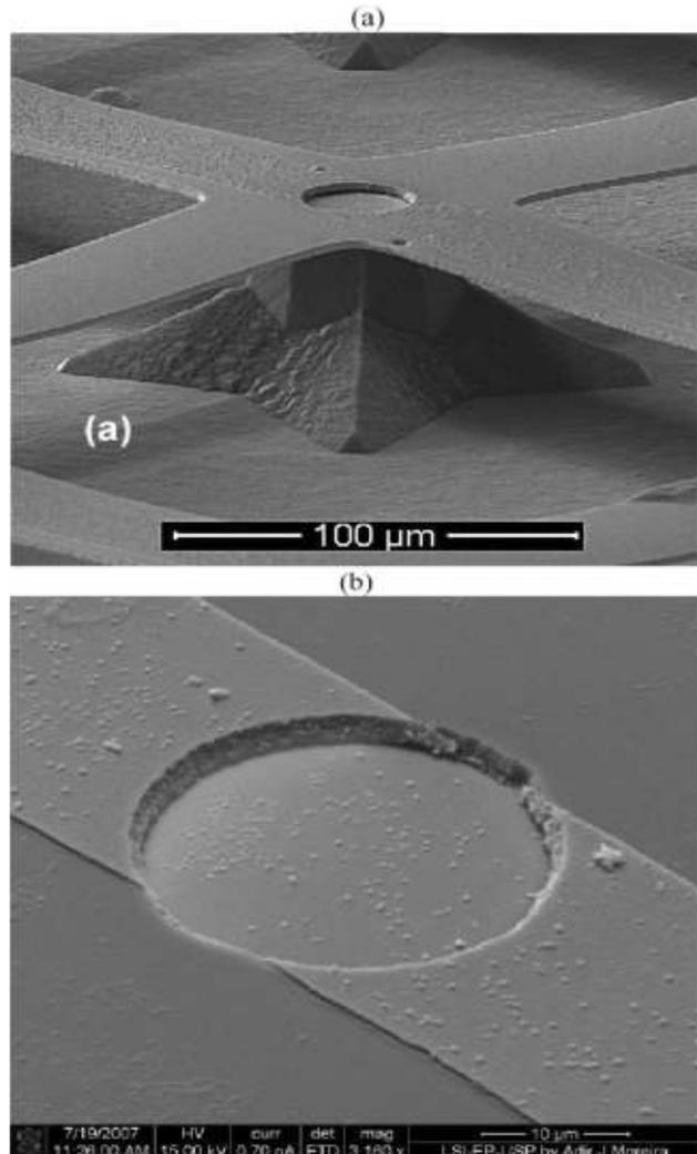
**Figure 9.** (a) Typical aspect of Cr electrode over the tips in the third stage of the tip formation. (b) Close-up of the circular region where the SiO<sub>x</sub>N<sub>y</sub> must be removed to permit the electron collection in field emission devices. Images from a scanning electron microscope.
