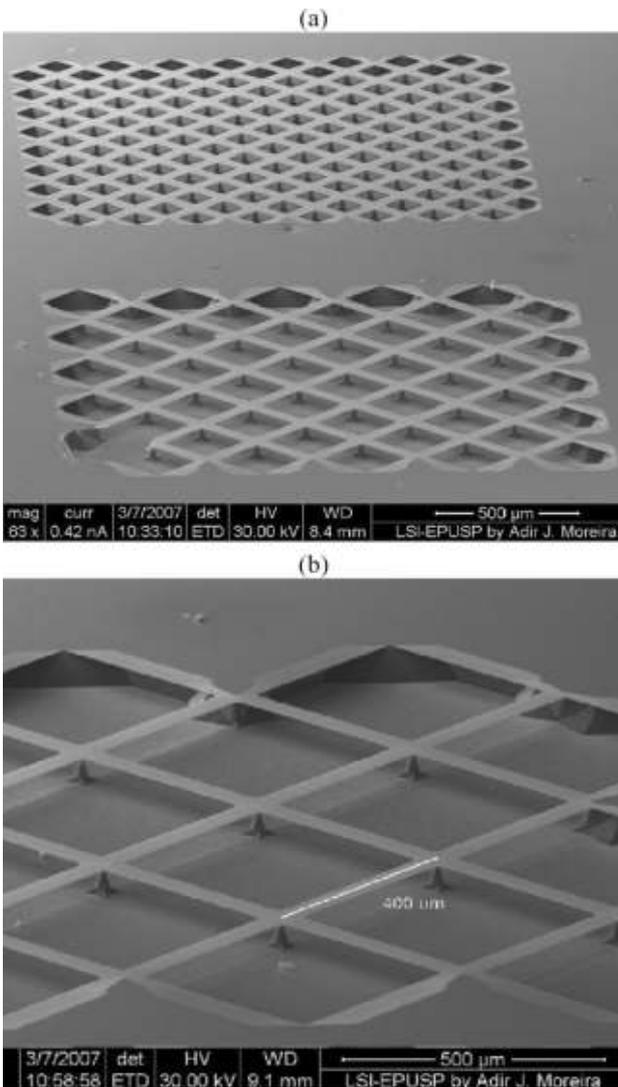
**Figure 6.** (a) Different matrices of microtips as viewed from a scanning electron microscope (SEM). (b) Detail of a microtip matrix formed from square holes of 400x400 µm<sup>2</sup>. Note the excellent structural integrity and flatness of the self-sustained SiO<sub>x</sub>N<sub>y</sub> grid.
