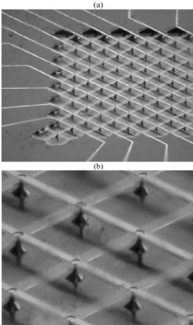
**Figure 8.** Final aspect of the Si microtips with the self-aligned integrated electrodes. (a) Matrix of 72 tips formed from square holes of 200x200 μm<sup>2</sup>. (b) Detail of the same structure. Images from an optical microscope.
