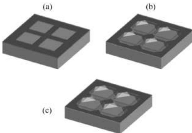
**Figure 2.** First stage of tip formation: (a) square holes in the masking material before the Si etching in KOH. (b) middle of the first stage, before the (100) walls collapse. (c) Formation of the isolated truncated pyramid marking the end of the first stage.
