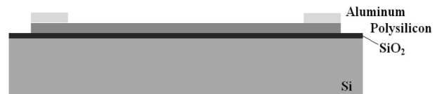
Figure 4. Schematic of the floating polysilicon resistor fabrication – Definition of the region aluminum pads.
