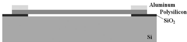
Figure 5. Schematic of the floating polysilicon resistor fabrication. Etching of sacrificial SiO 2 - Floating polysilicon resistor formed.
