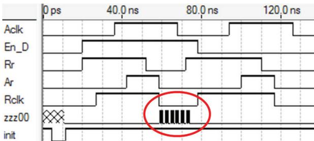
Figure 2. Simulation: input port of [21] presenting essential hazard
