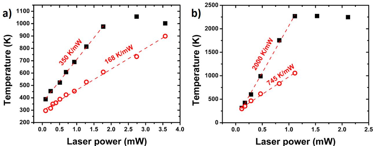
**Figure 3.** Laser heating of graphene on Au (a) and W (b) contacts. Dashed line (average slope) shows thermal resistance between contact surfaces.
