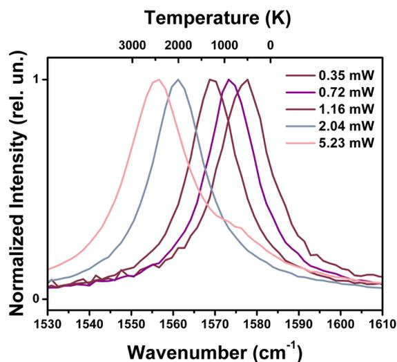
Figure 2. Shift of G-peak position caused by laser heating with different laser power for graphene flake deposited over W electrodes. Position of a maximum of G-peak corresponds to a temperature of the flake (shown on the top axis).
