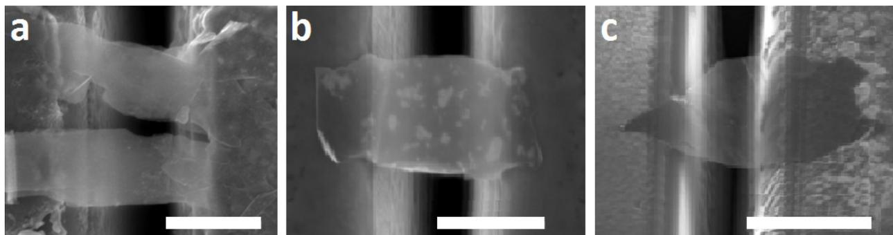
Figure 1. SEM images of multi-layer graphene flakes deposited over a) - W, b) - Ti and c) - Au electrodes. White bars correspond to 5  $\mu\text{m}$ .
