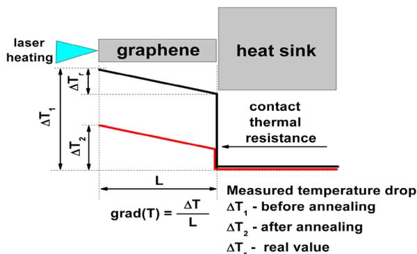
**Figure 4.** Schematics of the temperature distribution along the graphene before (black) and after the laser annealing of contacts with electrode.
