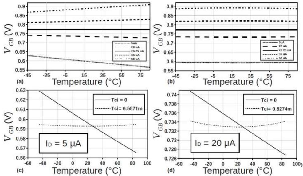
**Figure 2.** (a) simulations data for a diode-connected NMOS transistor ( $W/L = 2.5\mu\text{m}/1\mu\text{m}$ ) in 180 nm CMOS technology with five different bias current (5, 20, 26.25, 35, 50  $\mu\text{A}$ ), yielding distinct  $V_{GB}$  temperature dependence. (b)  $V_{GB}$  versus temperature enforcing right  $T_C$ , that cancels PTAT or CTAT behavior. (c) Zoom for  $I_D = 5\mu\text{A}$ . (d) Zoom for  $I_D = 20\mu\text{A}$ .
