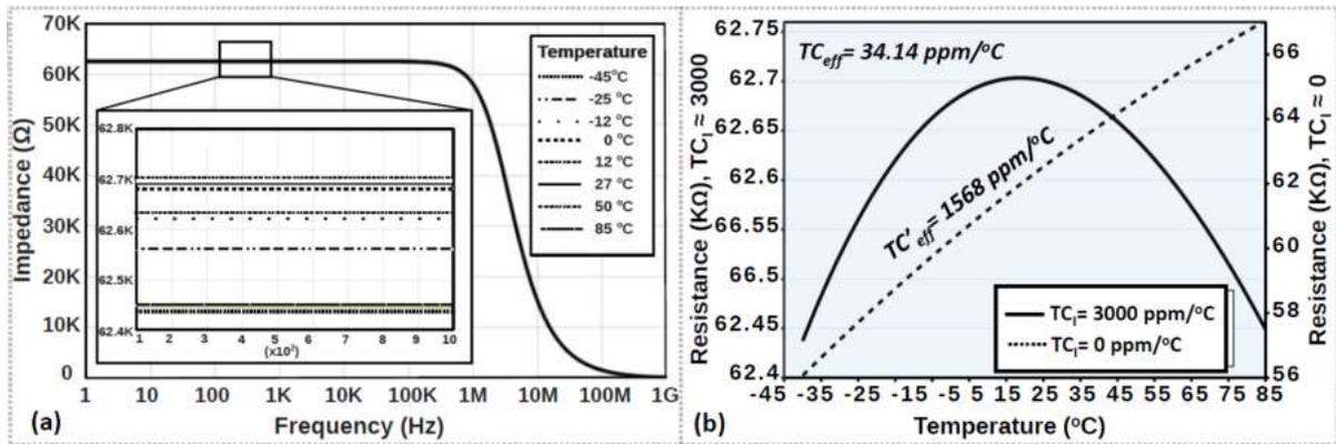
Figure 9. (a) Input impedance of single-ended resistor emulator (b) Equivalent Resistance vs. Temperature. Effective Temperature Coefficient is given by  $TC_{eff} = \frac{max}{(T_{max} - T_{min})} \frac{REF_{min}}{R_{REF}(T_0)} R_{REF} - R$
