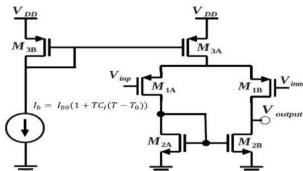
Figure 8. PMOS differential pair with active load.
