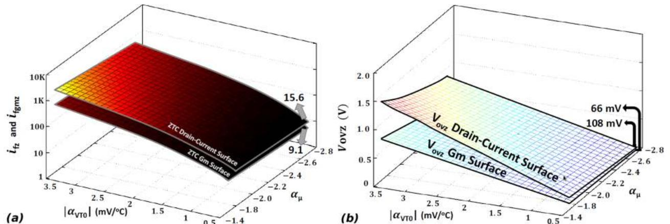
Figure 4. (a) ZTC forward inversion level surface (ZTCS) and GZTC forward inversion level surface (GZTCS) (b) overdrive voltage for the ZTC ( $V_{OVZ}$ ) and GZTC bias point ( $VOVGZ$ ) as a function of the values for  $\alpha_\mu$  and  $\alpha_{VT0}$ .
