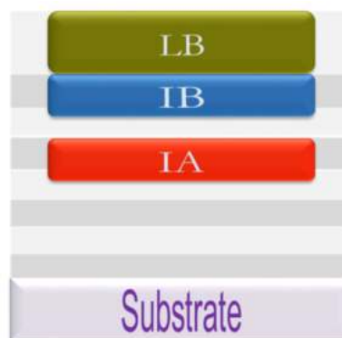
Figure 2. Cross-section of the top layers of the 28 nm BEOL (dimensions not to scale).
