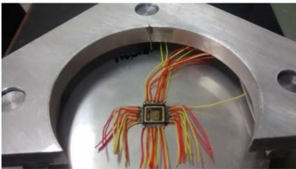
Fig. 8 Silicon device attached to metal disk substrate to be tested in Four-point bending apparatus.
