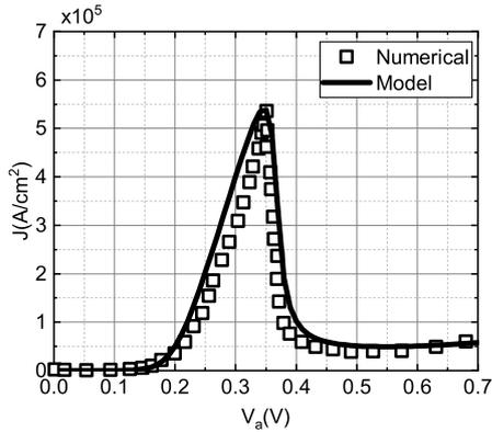
Fig. 5: Comparison between the  $I$ - $V$  curves obtained by the proposed current density model (solid curve) and the self-consistent numerical simulation (symbols) reported in [41].
