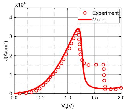
Fig. 3: Comparison between the **I-V** curves obtained by the proposed current density model (solid curve) and experimental data (symbols) of the RTD described in [25].
