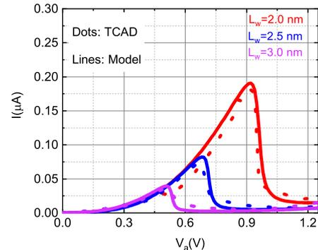
Fig. 8: Comparison between the  $I$ - $V$  curves provided by the proposed current density model (solid curve) and the quantum transport numerical simulation (dotted curve) obtained by TCAD simulation, for RTD #5, as a function of the well width  $L_w$ .
