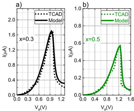
Fig. 10: Comparison between the I-V curves obtained by the proposed current density model (solid curve) and the TCAD simulation results (dotted curve) for RTD #7. a)  $x = 0.3$ . b)  $x = 0.5$ .
