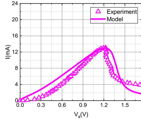
Fig. 4: Comparison between the **I-V** curves obtained by the proposed current density model (solid curve) and the experimental data (symbols) of the RTD reported in [40].
