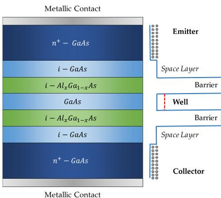
Fig. 1: Schematic illustration of a typical GaAs/AlGaAs Resonant Tunneling Diode layer sequence. Also shown it is a schematic illustration of the conduction band profile.
