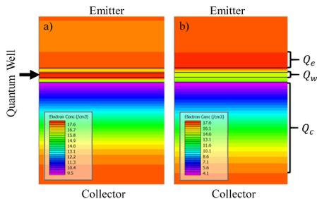
Fig. 7: Simulated 2D maps of the charge density for RTD #4. a) electronic concentration at the resonance peak. b) electronic concentration at the valley voltage range. The color change within the quantum well, from red to green, indicates a variation in the charge concentration, of about three orders of magnitude.
