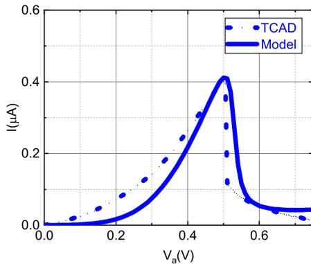
Fig. 6: Comparison between the  $I$ - $V$  curves obtained by the proposed current density model (solid curve) and the quantum transport numerical simulation (dotted curve) carried out using the Atlas Silvaco TCAD software.
