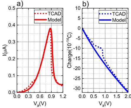
Fig. 9: Comparison between the results obtained by our proposed model (solid curves) and the TCAD simulation results (dotted curves) for RTD #6. a) I-V characteristics. b) emitter charge.
