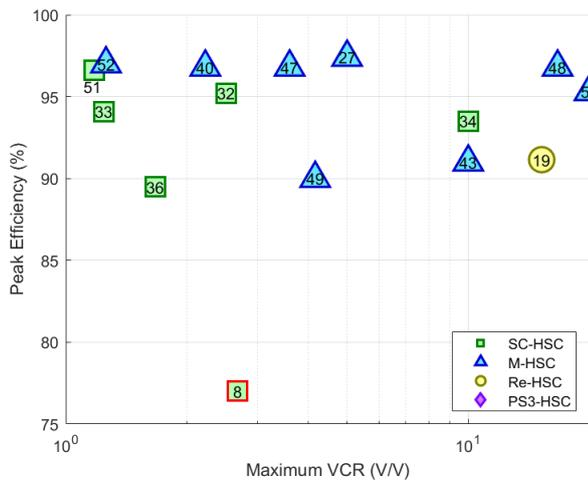
Fig. 17. State-of-the-art form HSCs: Peak efficiency vs. maximum VCR: step-up conversion.
