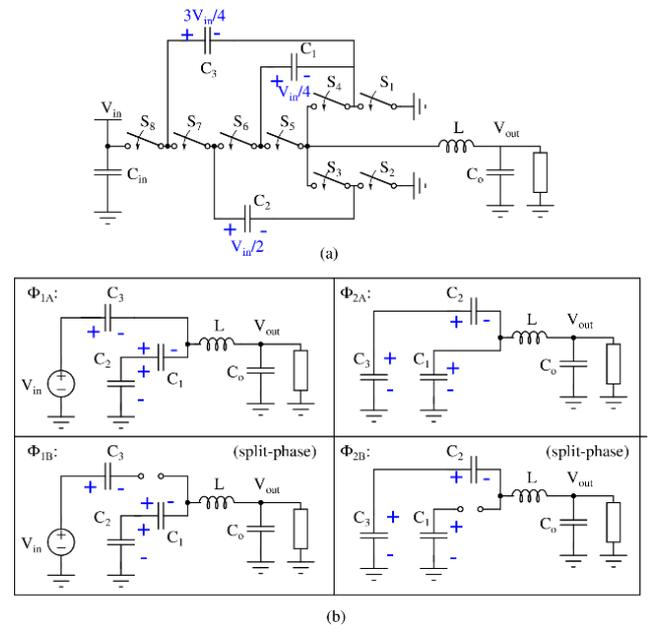
Fig. 8. Dickson based M-HSC: (a) basic structure and (b) operation phases. Adapted from [6]
