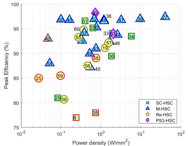
Fig. 14. State-of-the-art form HSCs: Peak efficiency vs. Power density.
