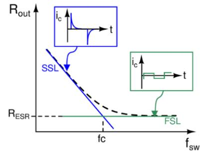
Fig. 1. Output resistance vs. Switching Frequency [16].
