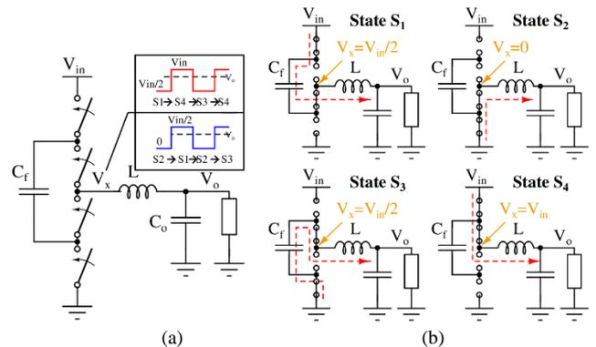
Fig. 7. 3-level step-down M-HSC: (a) basic structure and (b) operation states.
