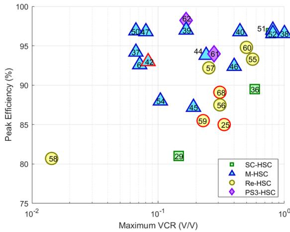
Fig. 16. State-of-the-art form HSCs: Peak efficiency vs. maximum VCR: step-down conversion.
