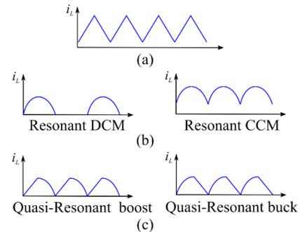
Fig. 10. Inductor current waveform: (a) SIC, (b) DCM and CCM resonant, (c) quasi-resonant.
