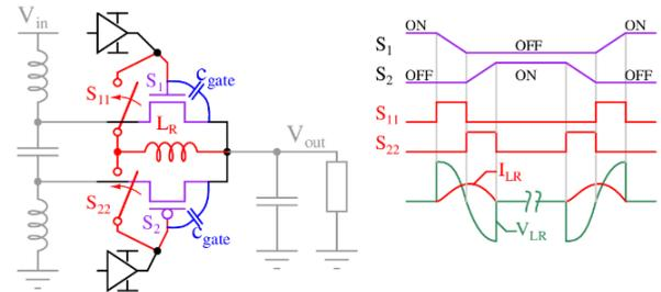
Fig. 13. Charge-recycling in PS3-HSC. Adapted from [62].
