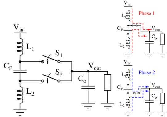
Fig. 12. Passive-stacked 3<sup>rd</sup>-order HSC (PS3-HSC). Adapted from [61]
