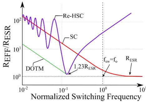
Fig. 9. SCC and Re-HSC output resistance. Adapted from [67]
