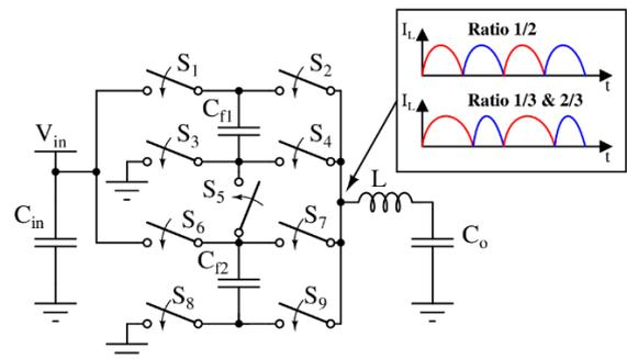
Fig. 11. Fully-integrated Multi-ratio Re-HSC. Adapted from [25]
