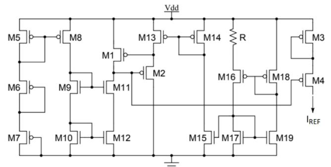
Fig.14 Current reference proposed by [18].
