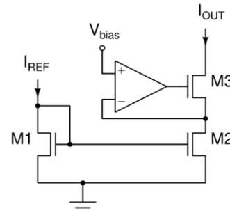
Fig. 7 Enhanced output-impedance current mirror.
