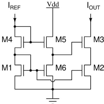
Fig. 5 Modified cascode current mirror.
