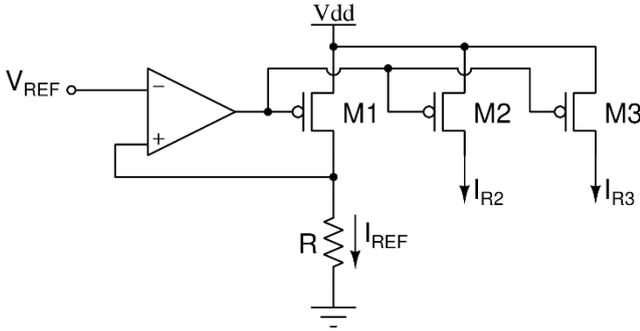
Fig. 10 Current reference using Op.-Amp.
