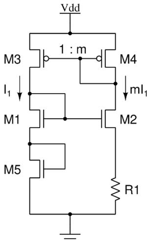
Fig.15 Current reference proposed by [19].
