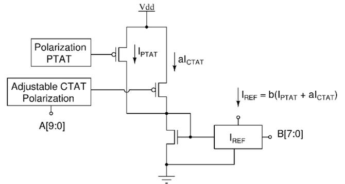
Fig. 16 Current reference proposed by [20].
