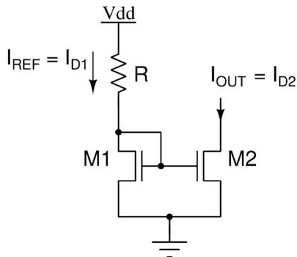
Fig. 8 Simple current reference.
