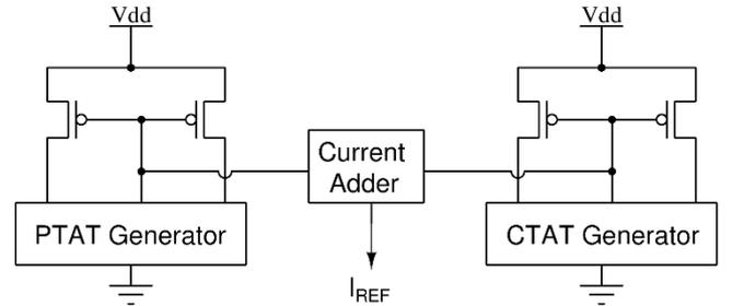
Fig. 13 Generic current reference circuit
