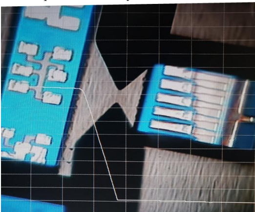
Figure 2. Profilometer measurement of SU-8 thickness.
