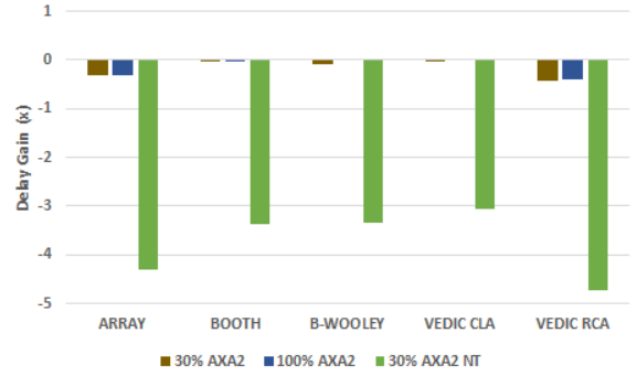
Fig. 15: Delay gain of AXA2 approaches compared to the nominal scenario using the LP model
